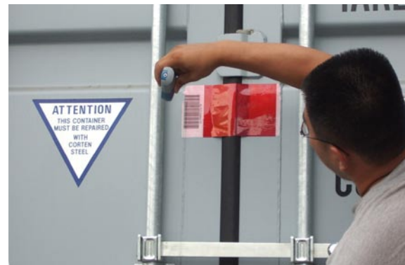
Handheld computer reading barcode for container identity check
